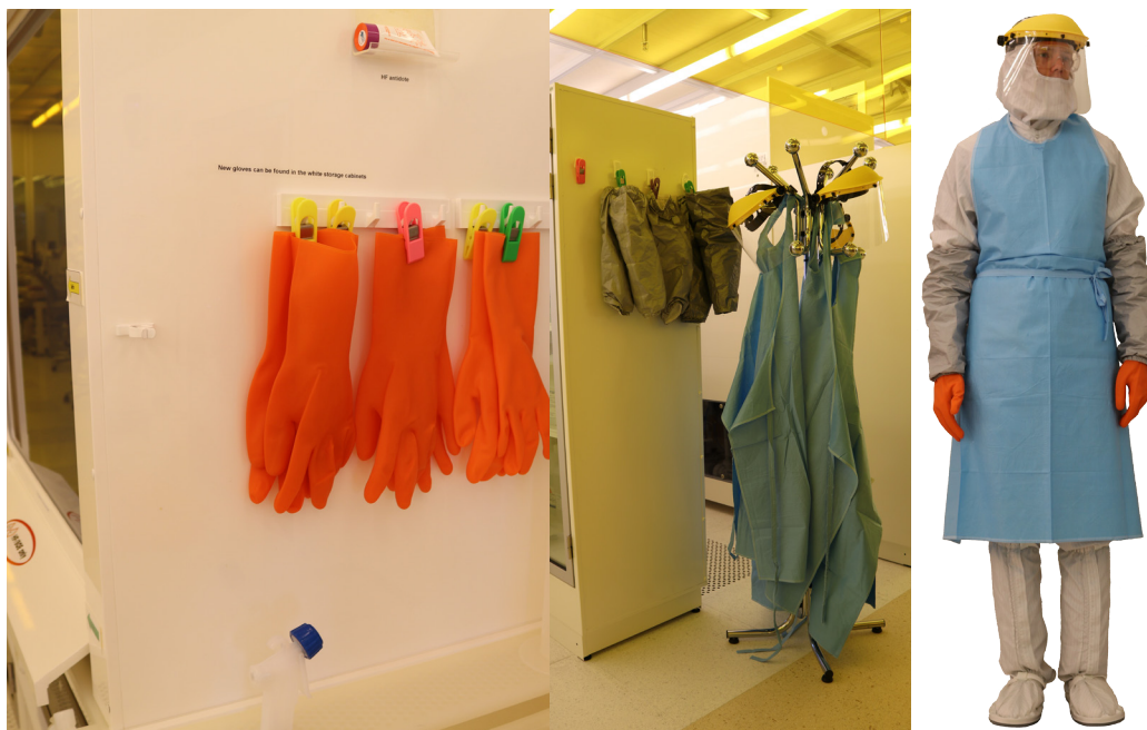
Figure C3: First two pictures showing the hangers for protective gear; gloves, face shield, apron and arm cover. Fully equipped chemical protection seen to the right.
